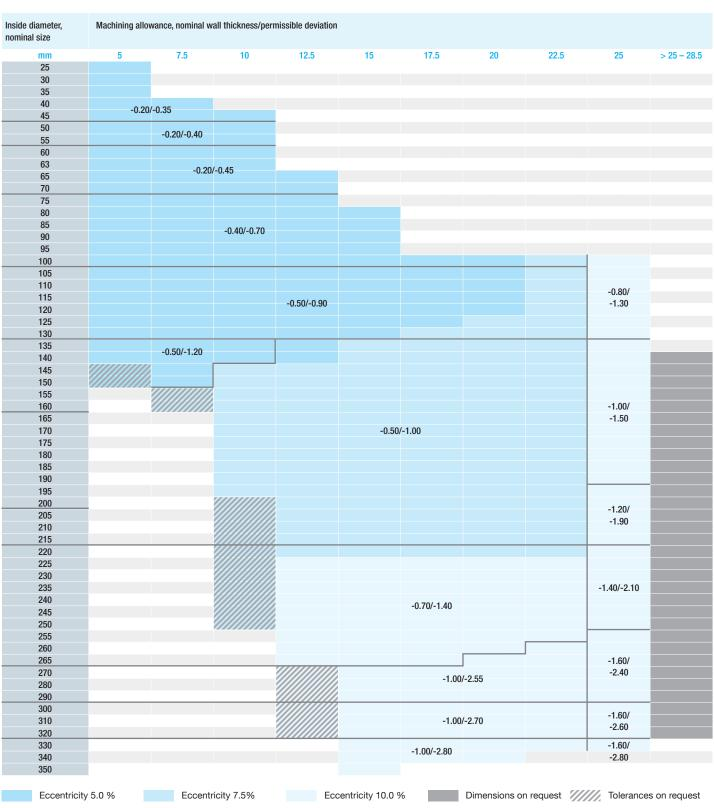
Tubes for cylinder construction are seamless cold finished precision steel tubes in the delivery conditions +N or +QT, or tubes in the delivery condition +SR outside the specified size or tolerance ranges for the manufacture of cylinder barrels.
